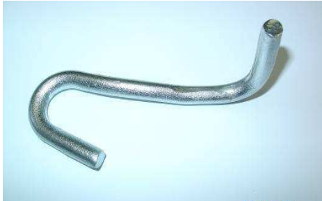
Figure 13: Straightened hook after test carried out.
