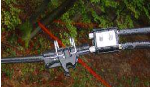
Figure 12: Special spring clamp after test carried out
